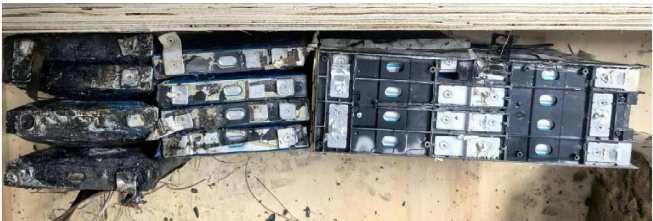
Damage of the internal components
