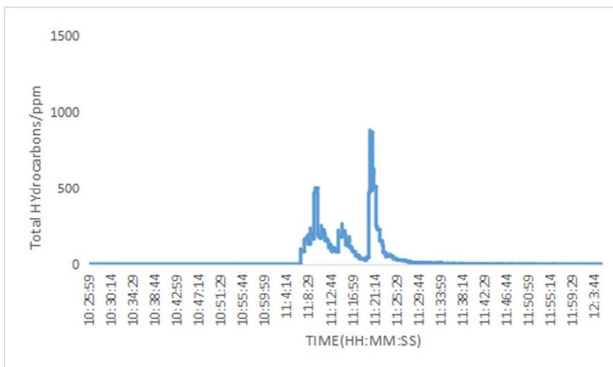
Figure 14. Total Hydrocarbons (equivalent to C<sub>3</sub>H<sub>8</sub>, measured by FID)
