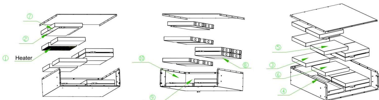
Remark: The number 1~10 means Thermocouple no. T1~T10 distributed in modules.
