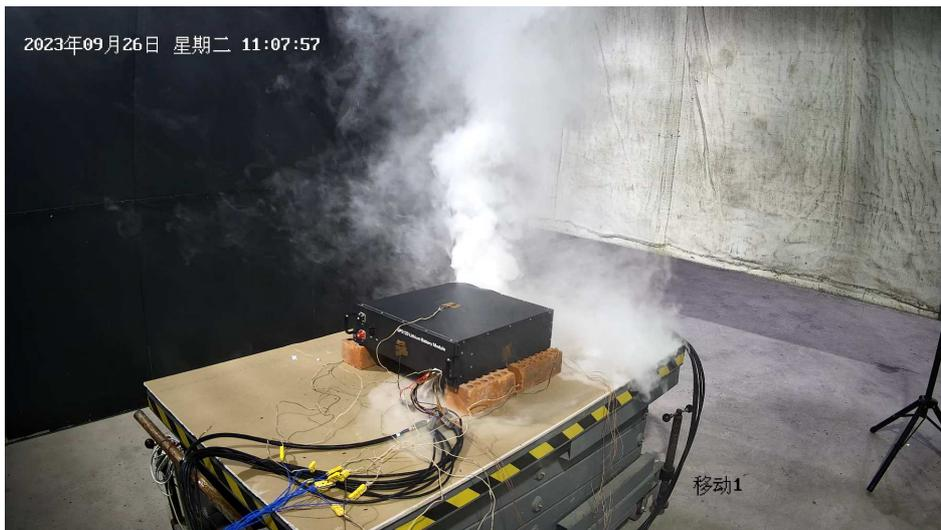
Smoke release during test
