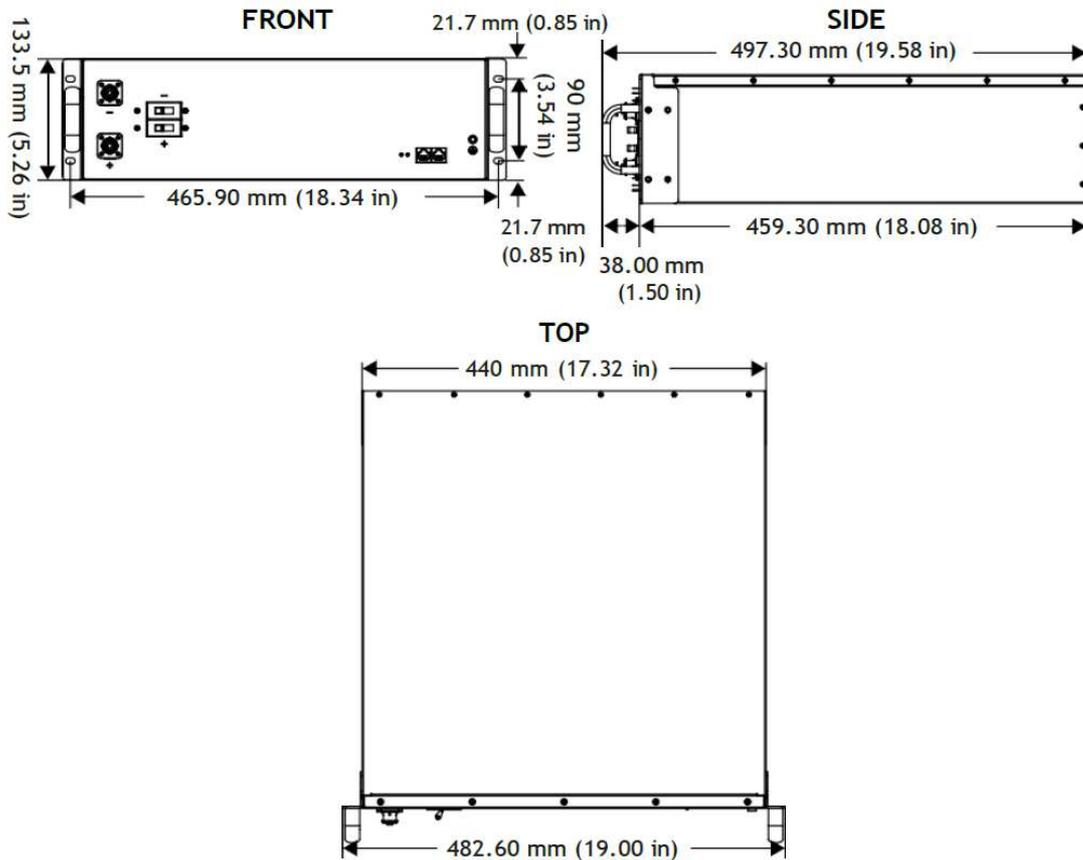
Figure 1. Diagram with overall dimension (Unit: mm)
