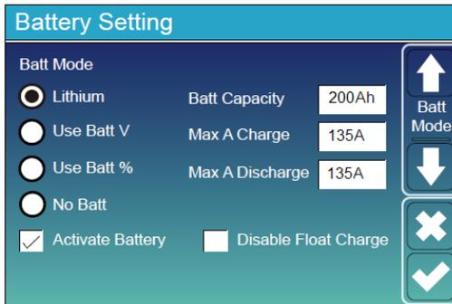
**Figure 6. Battery Setting - Closed-loop Charge Settings**
