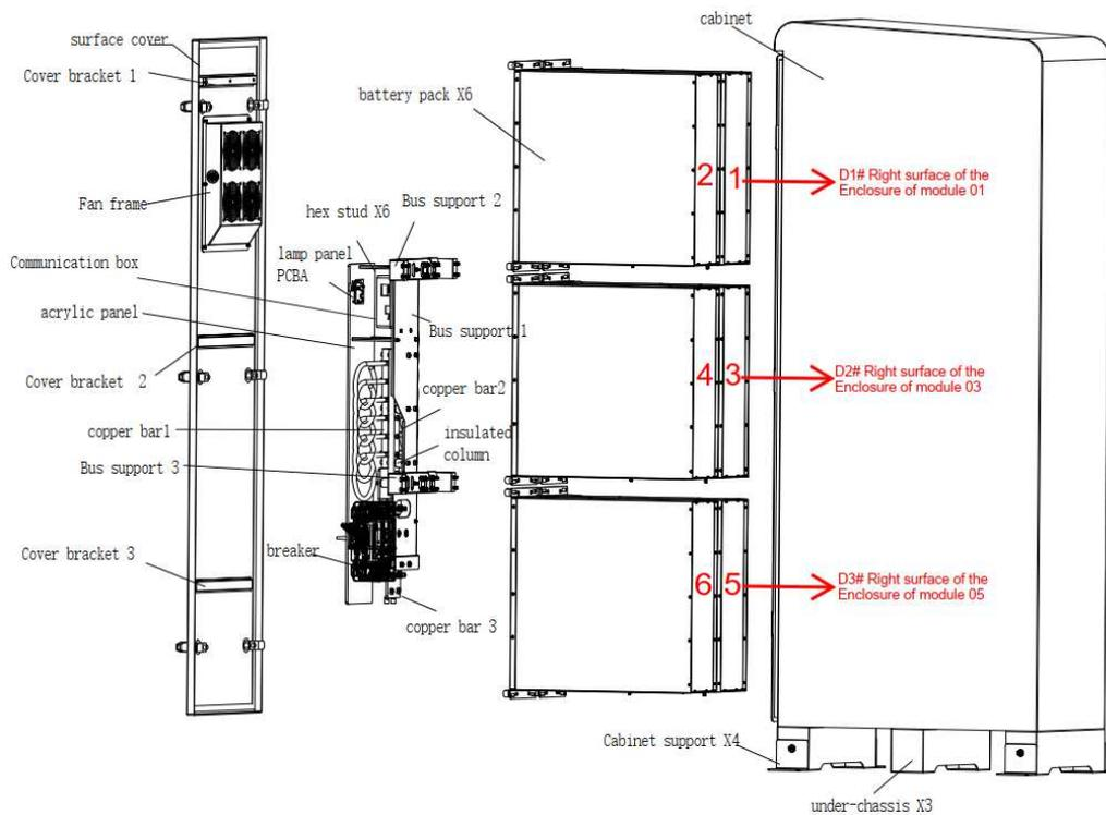
Figure 4. Thermocouple in target unit 01
