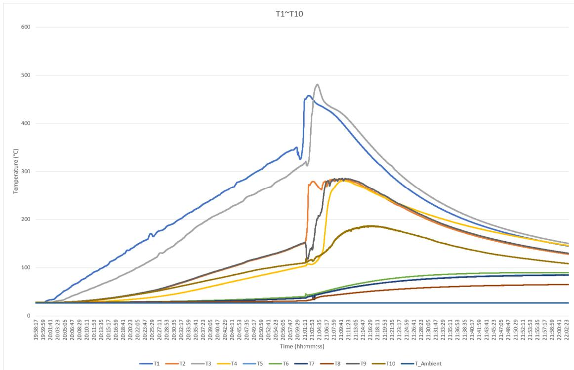
Figure 8. Temperature vs time curve of module 04 in initiating unit.
