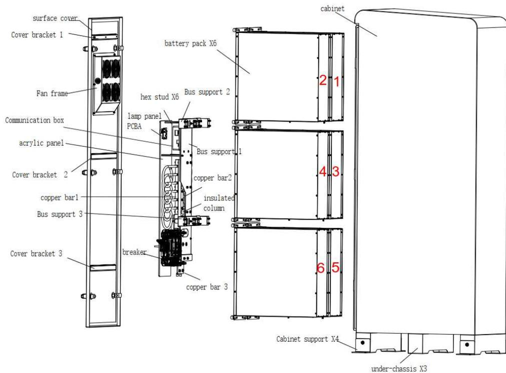
Figure 2. Module numbering in unit
