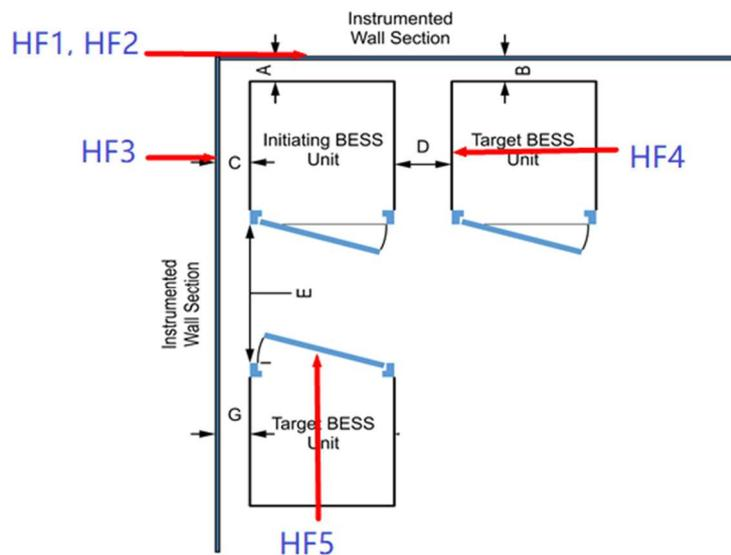
Figure 11. Heat flux sensor layout
